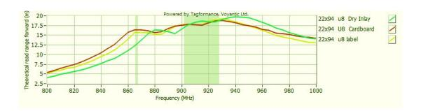
Sensitivity&Read Range Test power: 4W EIRP
